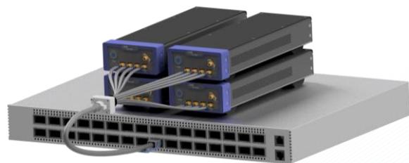
Figure 3 Switch Testing using 4 Pulsars.
