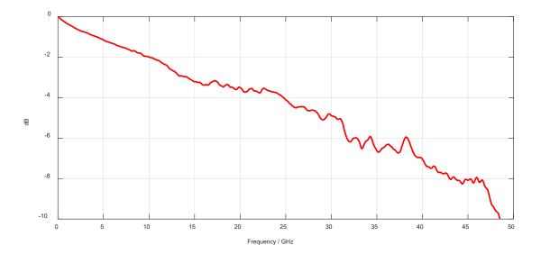
Measured Insertion Loss data of 800G QSFP-DD Adapter:
