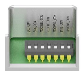
Each low-speed signal can be controlled independently from the next. To switch each of the low-speed signals sources, it suffices to slide its' switch to the top or bottom side.
