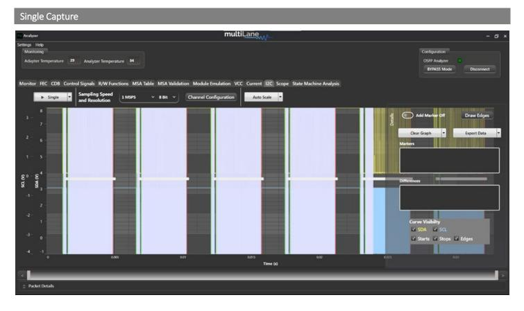
I2C Single, trigger and tracking captures show SDA, SCL, Start, Stop and Edges on the graphs.
