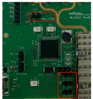
Figure 2: External Control Signals
