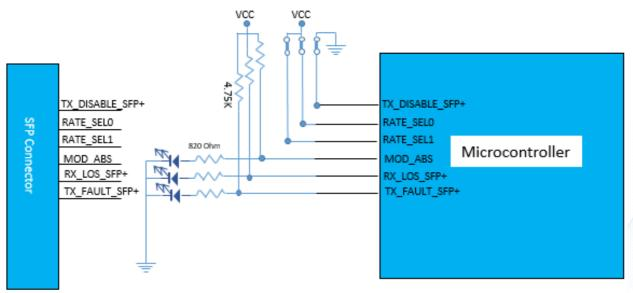
Figure 3: Low Speed Signals Schematics
