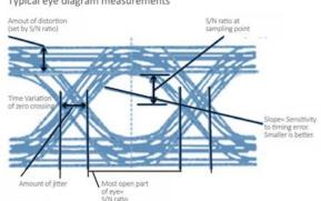
*Figure 1: Jitter and noise effect on eye shape*
