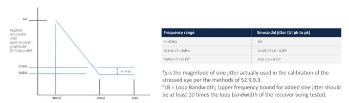
Figure 3: IEEE 802.3 SJ Injection Mask
