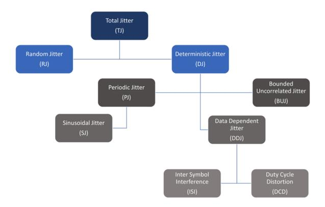
Figure 2: Breakdown of jitter components
