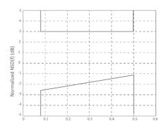
*Figure 5: Spectral flatness per IEEE 802.3ck specs*
