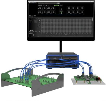
Figure 21: Electrical Rx transceiver testing setup
