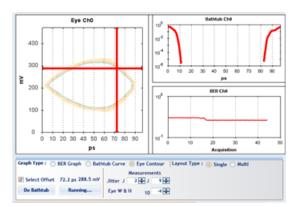
Figure 25: Single Channel Eye Contour
