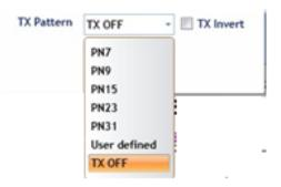
Figure 7: PRBS Channel Configuration
