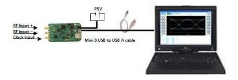
Figure 24: Connection via USB
