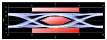
The DSO has these standard masks: 100Gbase-SR, LR, STM-1, STM-4, STM-16, Gb Ethernet, Fiber Channel (1x), Fiber Channel (2x, 4x), Fiber Channel (8x), Fiber Channel (10x), 10 Gb Ethernet, and user defined masks. New masks are continuously added. Recent additions are QDR & FDR.
