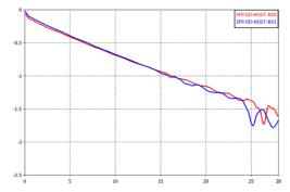
Figure 1: ML4022-MCB Insertion Loss
