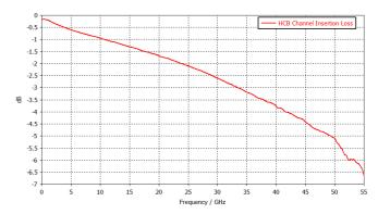
Figure 3: ML4064-HCB-112 Insertion Loss
