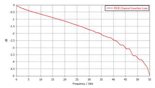
Figure 1: ML4064-MCB-112 Insertion Loss
