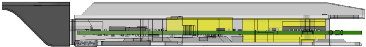
Figure 7: Thermal Interfaces Distribution
