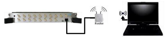
Figure 32: ML4039 connected to PC via Wireless
