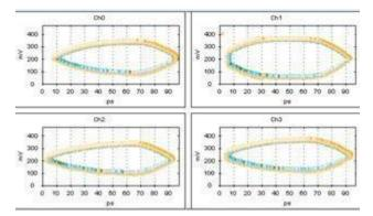
Figure 26: 4 Channels Eye Contour
