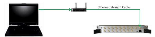
Figure 31: ML4039 connected to PC via Ethernet
