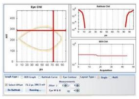
Figure 25: Single Channel Eye Contour
