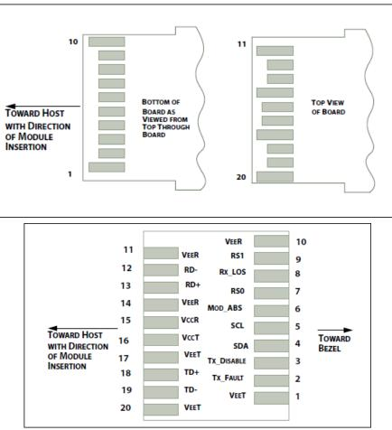
Figure 7: SFP56 Module Pin Map
