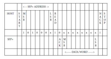
Figure 1: SFP56 Current Address Read Operation
