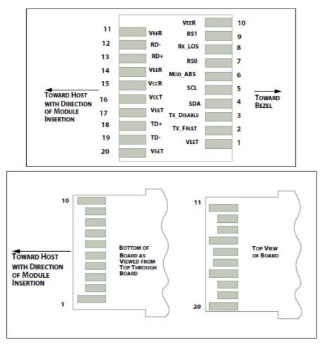
Figure 7: SFP28 Module Pin Map
