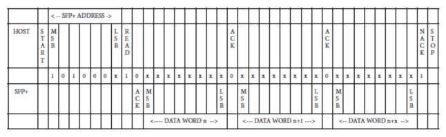
Figure 1: Sequential Address Read Starting at SFP28 Current Address
