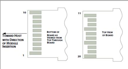
Figure 7: SFP Module Pin Map
