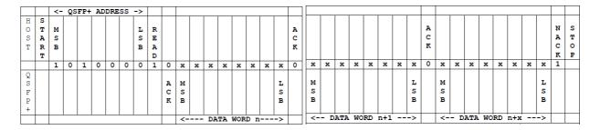
Figure 4: Sequential Address Read Starting at QSFP+ Current Address
