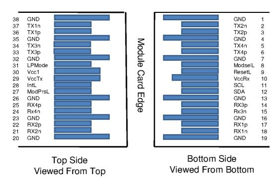
Figure 6: QSFP+ Module Pin Map
