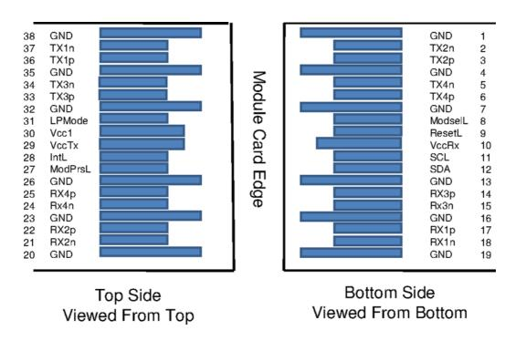
Figure 6: QSFP Module Pin Map
