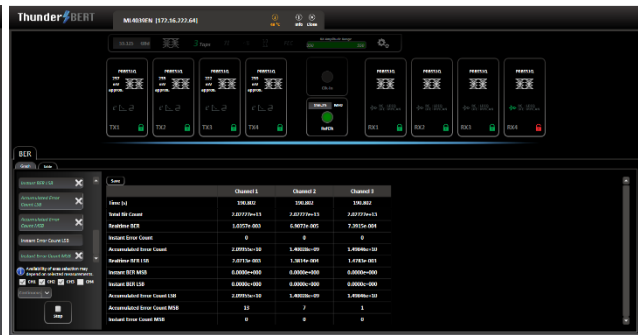
Figure 36-2: BER table measurements
