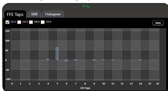
Figure 29: Rx diagnostics FFE Taps
