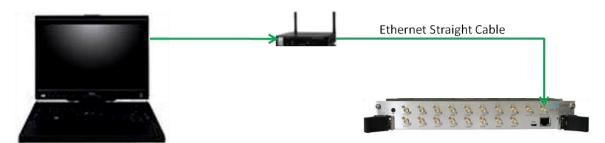
Figure 24: ML4039B/-JIT/-EQL connected to PC via Ethernet
