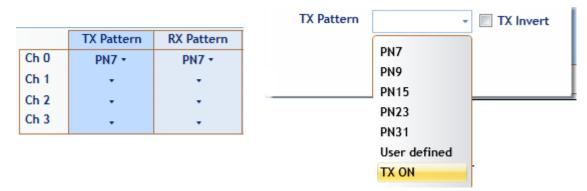
Figure 7: PRBS Channel Configuration
