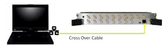
Figure 25: ML4039B-EQL connected with Ethernet crossover cable
