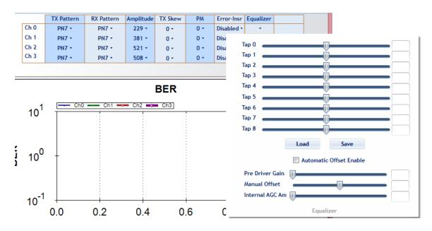
The tabs contain predefined IEEE stress conditions; The FFE (Feed Forward Equalizer) taps can shape the output signal according to the taps values. They provide superior modal dispersion compensation and enable full control of the signal.
