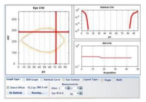
Figure 18: Single Channel Eye Contour
