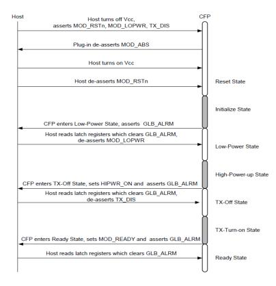
MOD\_RSTs assertion drives the CFP2 module to a reset state, at this stage the MDIO interface will be held in a high impedance state, the Host will read 'FFFF'h from any address, while host write operations will have no effect.
