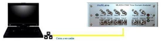
Figure 33: ML4004-PAM connected with Ethernet crossover cable
