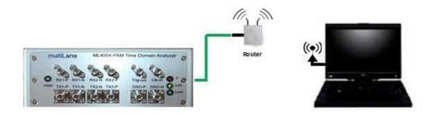
Figure 34: ML4004-PAM connected to PC via Wireless
