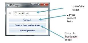
Press connect twice, start in boot loader mode, you will be redirected to the PIC 32 tool.
