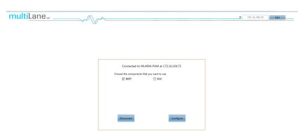
When you enter the IP address and connect to the instrument, you are presented with the above menu. Choose if you plan on using the ML4004-PAM as BERT only, Scope only or both.
