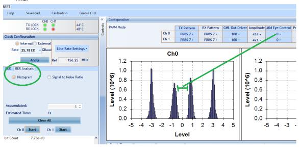
In the histogram above, you see that the inner eye is smaller than the upper and lower eyes. To change this ratio, go under the Mid eye control tab and change the value then repeat the histogram scan.
