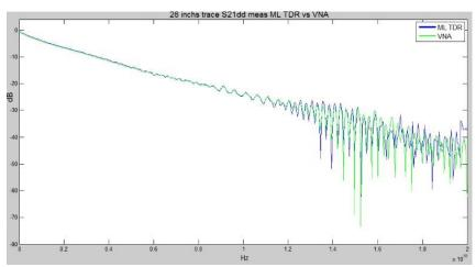
Figure 32: Comparison of performance and accuracy between a 40 GHz VNA and the ML DSO
