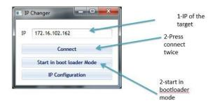
Press connect twice, start in boot loader mode, you will be redirected to the PIC 32 tool.
