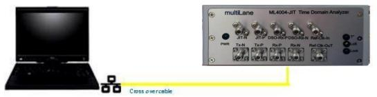
Figure 40: ML4004-JIT Rev B connected with Ethernet crossover cable
