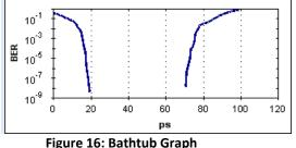
Plotting the points on a graph of BER versus sampling location in time results in curves as shown in Figure 13. A bathtub curve can be created either by software extrapolation from voltage over time measurements done by an oscilloscope, or by actually sampling the bits as done by a BERT.
