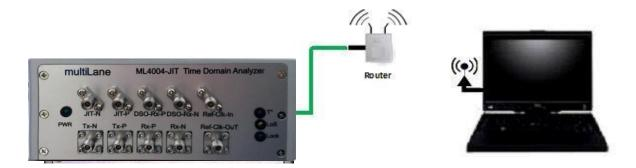
Figure 41: ML4004-JIT Rev B connected to PC via Wireless
