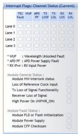
Figure 46. Interrupt flags: Channel Status (Current)
