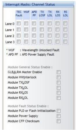
Figure 66. Interrupt Masks: Channel Status
