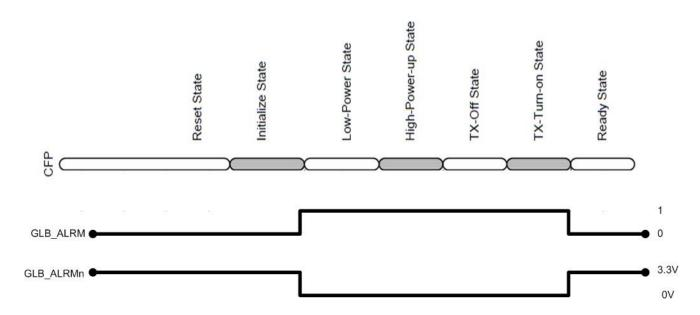
GLB \_ALRM is de-asserted during Reset and Initialize state, it is asserted in Low-Power,High-Power-up, Tx-Off and TX-Turn-on states, then de-asserted again when ready state is reached. GLB\_ALRMn is the hardware pin, and is the inverse of GLB\_ALRM.
