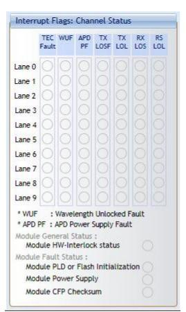
Figure 19 Interrupt Flags: Channel Status Window
