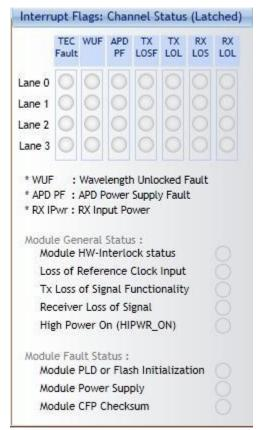
Figure 50. Interrupt flags: Channel Status (Latched)
