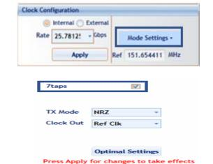
After applying the settings, the seven-tap control will be available for editing under the amplitude menu. Any one of the 7 taps can be defined as main tap; in this case, taps preceding it will be precursors. Likewise, taps following the main tap will be post-cursors.
