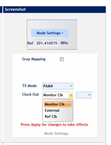
To switch between NRZ and PAM-4 coding, use the TX Mode setting, then click Apply.
