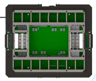
Figure 1: Four ML cassettes mounted in an Advantest V93K HSIO test head extender frame
