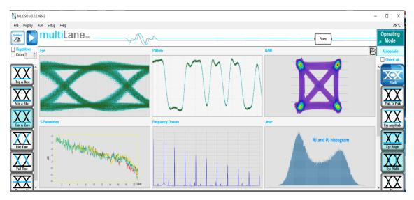
Figure 12: Supported DSO GUI Operating Modes
