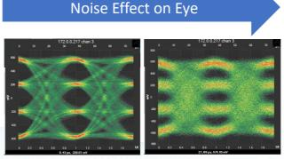
Figure 9: Eye Diagram before and after noise injection – PAM4 modulation
