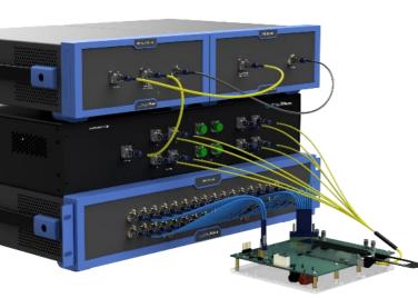
Quad WDM transceivers up to 400G use the MLO4034-CWDM4 or LR4 variant, while Octa WDM transceivers use the MLO4034-LR8 variant.
