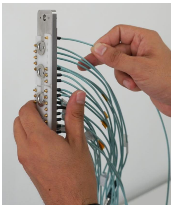
Figure 6. Inserting Cables. Nuts on backside
