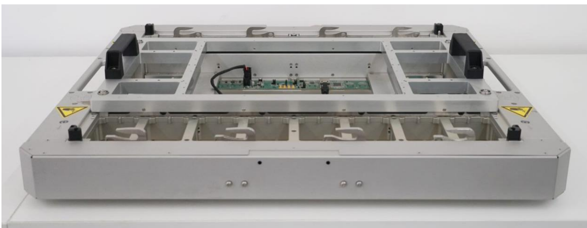
Figure 2. Diagnostic Stiffener Hard Docked
