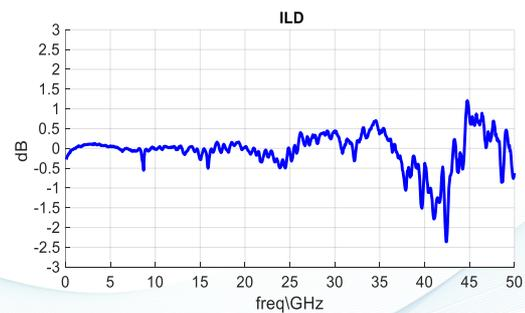
Insertion loss deviation up to 50 GHz
