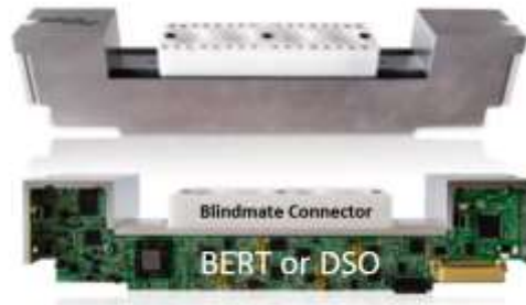
Figure 4: AT93000 Cassette with exposed instrument
