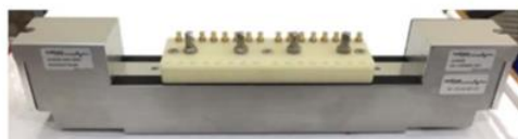
Figure 3. MultiLane instruments are packaged in cassettes for insertion into the HSIO card cage.
