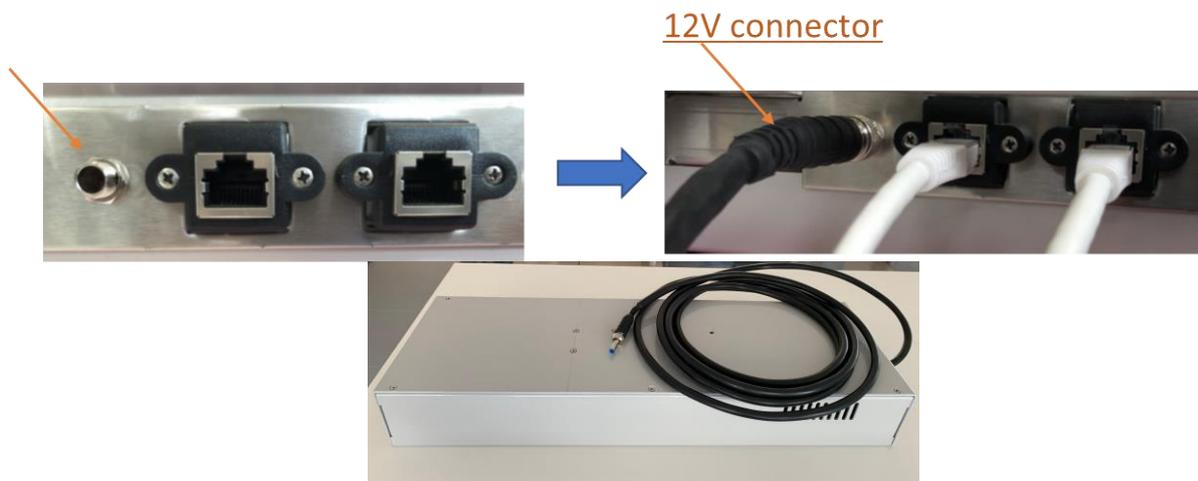
Figure 25: AT93000 Power Supply
