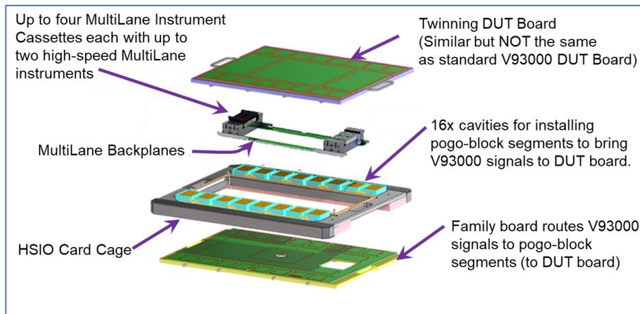
Figure 2: Building blocks of the Multilane AT93000 system
