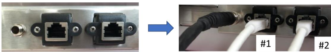
Figure 29: Ethernet Connectors Associations with each Backplane
