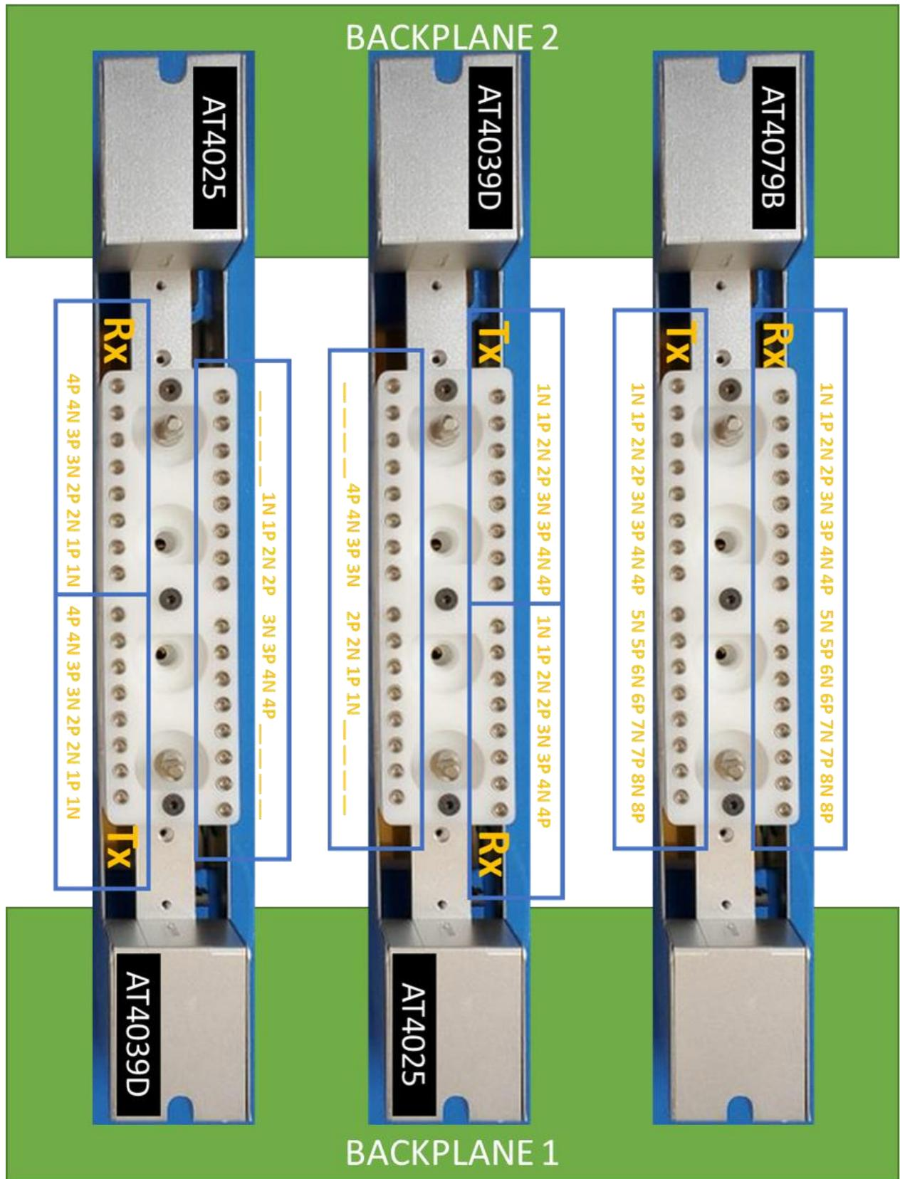
Figure 12: Pinouts for different cassette rotations plugged into backplane 1 or 2
