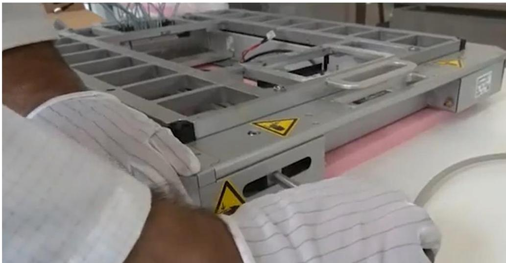
Figure 27: Manual docking of DUT loadboard to AT93000 twinning frame
