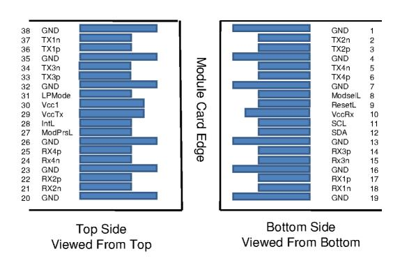
Figure 6: QSFP+ Module Pin Map
