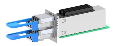
Figure 2-8: Two type 2B modules shown in a QSFP-DD800 stacked cage. Note the alignment of the faceplate and cage openings coincide with the nose heatsink channels
