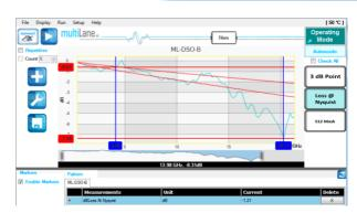
Figure 2: Adaptive channel equalization for up to 14dB loss at Nyquist
