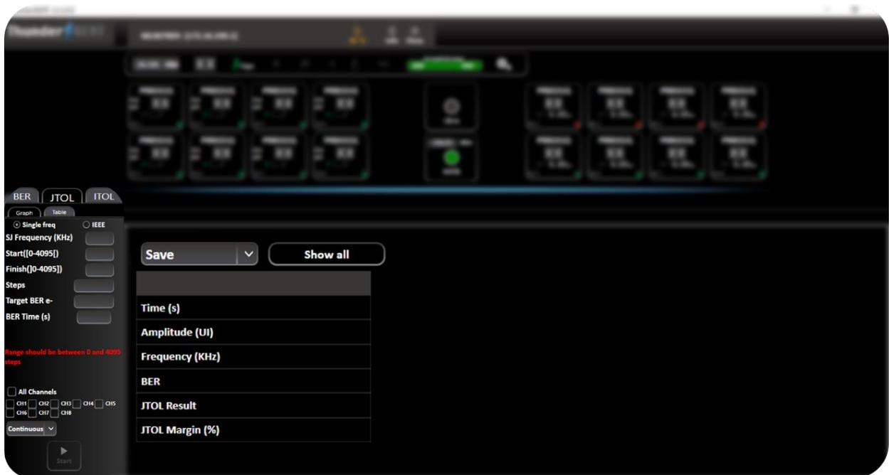
Figure 10: Single frequency JTOL control and results table
