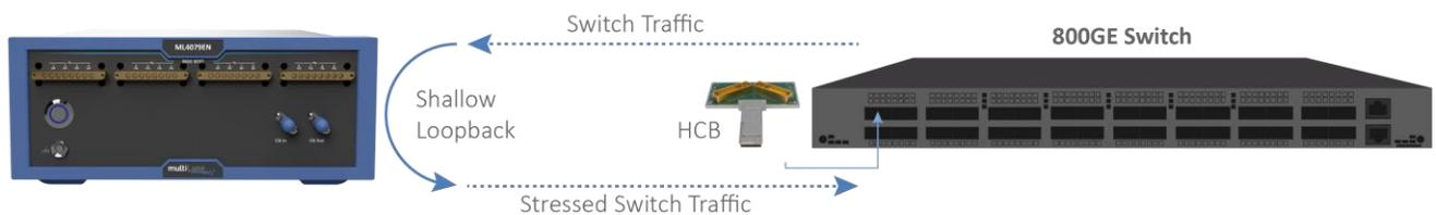
Figure 17: Shallow loopback testing setup
