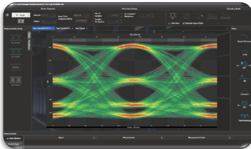
Figure 6: Adjusting different inner/outer eye levels
