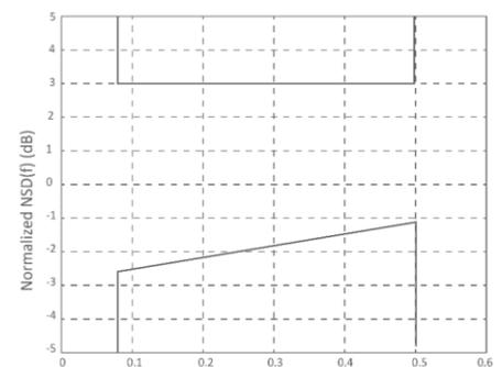
Figure 5: Spectral flatness per IEEE 802.3ck specs
