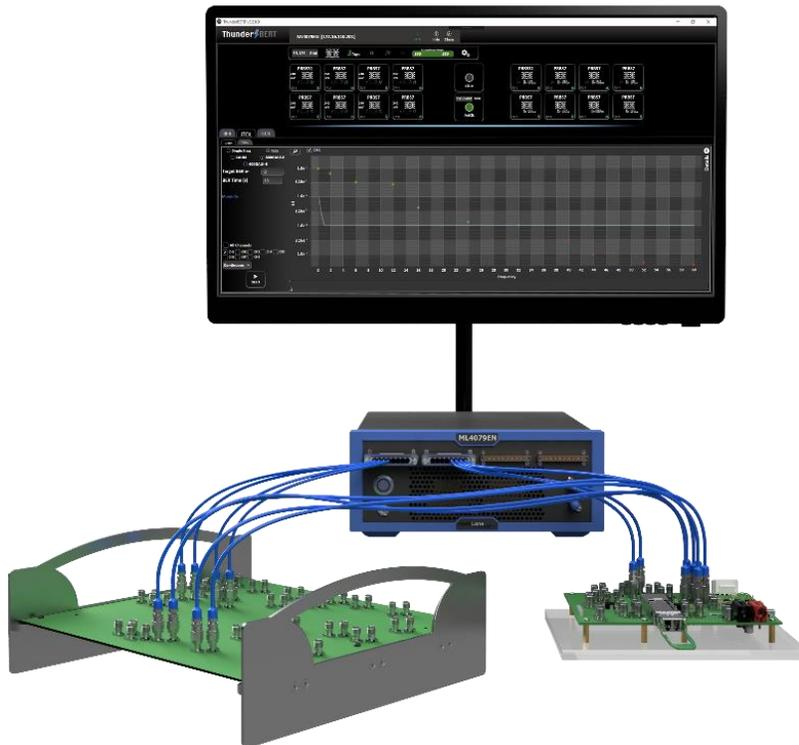
Figure 21: Electrical Rx transceiver testing setup
