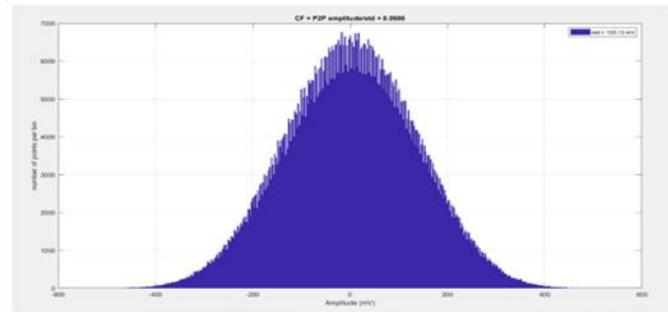
Crest Factor Measurement: Gaussian Noise
