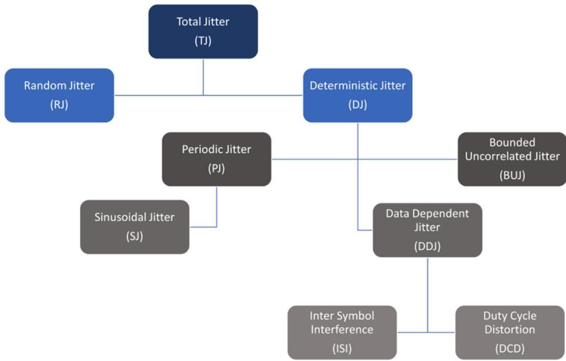
Figure 2: Breakdown of jitter components
