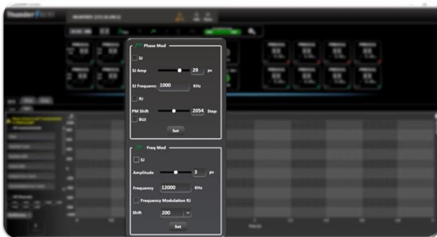
Figure 8: MultiLane supported jitter types
