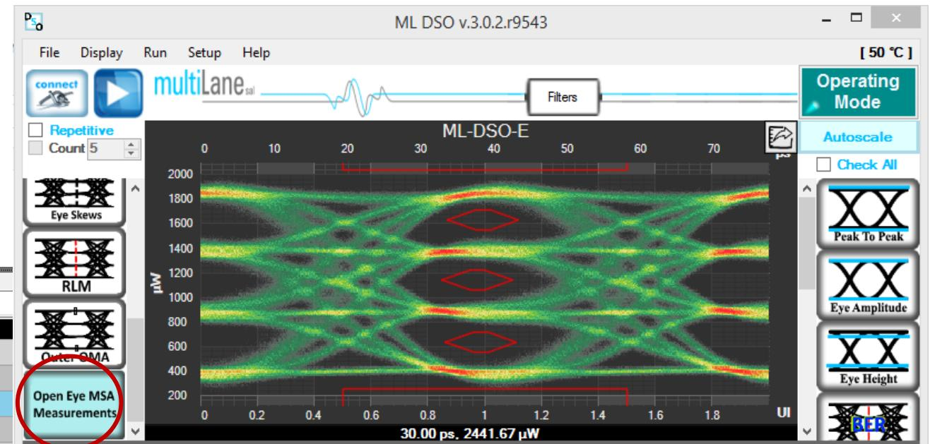
Measurement tab to select Open Eye specific measurements.
