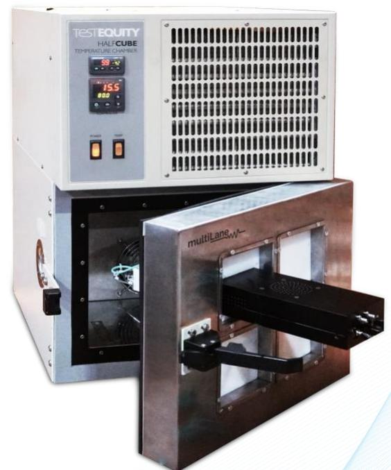
Figure 6: Low profile ML4054-400, mounted on custom oven door (MLT8000)
