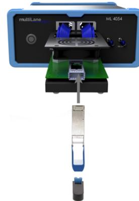
As this BERT is also equipped with a 400G host interface, a user can force a DUT (OSFP or QSFP-DD) into a preferred operating condition, which would in this example be FEC Bypass Mode. After setting transmit characteristics within **ThunderBERT** and connecting a fiber loopback to the module, a sample of supported test operations follows:
