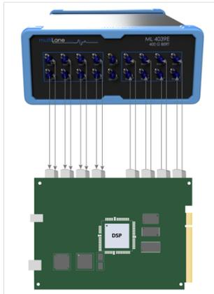
This application enables characterization of host-side DSP performance in a benchtop setting. A user can set a desired line rate, PRBS pattern and equalization taps in the **ThunderBERT** configuration window and execute the following sample measurements while cycling the DUT through various operational modes:
