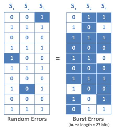
Primary noise sources that can attribute to random errors include fluctuations in the DC power level delivered to active components along with the cross talk and insertion loss that occur due to marginal signal integrity from wire bonding. While the limitations of lossy signal traces are indeed compensated by a variety of equalization techniques, the techniques themselves can be responsible for the large strings of errored bits we identify as bursts.
