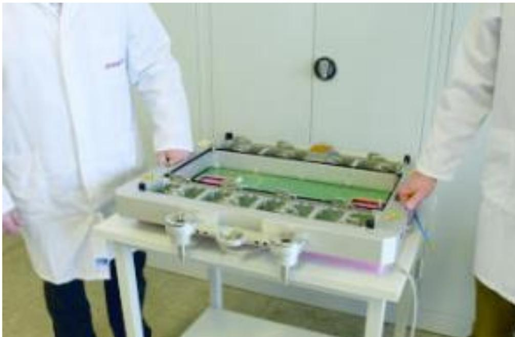
Figure 4: MultiLane Card Cage (also called "Twinning Frame")
