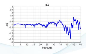
Insertion loss deviation up to 50 GHz
