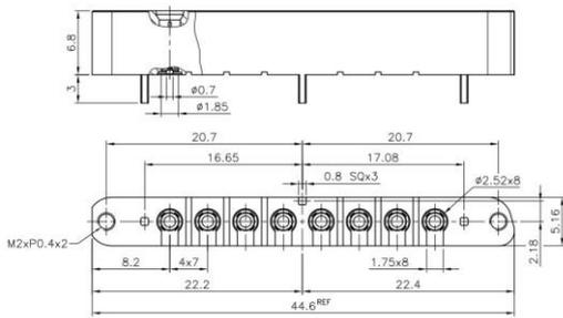
Figure 5: PCB connector drawing
