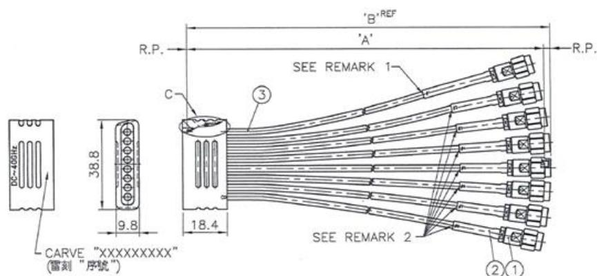
Figure 3: Cable assembly – Type A M-SMPM to K-connector
